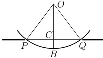
Figure 3.45: The Spherometer
