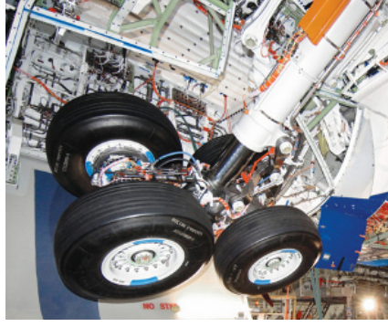
Figure 1: Hundreds of flexible conduits in the landing gear of an airplane.
